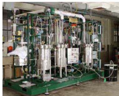
Figure 14. The Department's greatest contribution to Louisiana is the practical training it has provided thousands of ChE's. In the last 10 years it has made capital improvements of more than $4 MM (in partnership with industrial donors) to modernize its undergraduate labs. Shown here is a polymerization reactor/separator experiment brought on-line in 2000. It was designed and assembled under the direction of Paul Rodriguez, who has made ours among the best Engineering shops in the nation.
