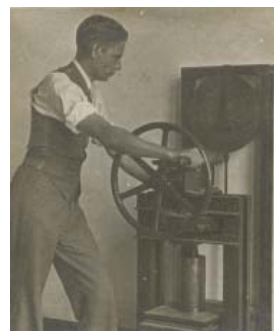
Figure 11. William Richardson (M.S., 1932) testing compressive stability of a mineral aggregate / asphalt mix for the Louisiana Highway Chemical Testing Lab. LSU did not offer Ph.D. degrees until the early 1930s, and most of the early M.S. projects were tied to the sugar, naval stores, paper, oil refining, natural gas and asphalt industries [1-7]. All of this work was funded by Louisiana industries and tied to their improvement.
